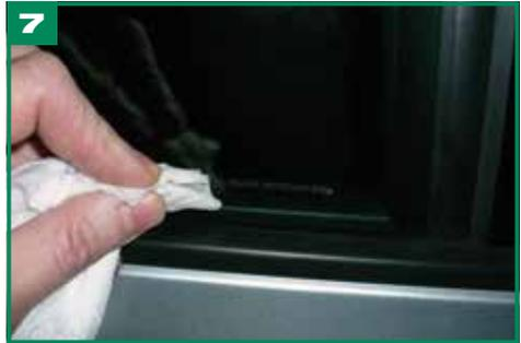
Etched VIN clean with wet cloth and instantly remove any leftover acid gel on glass.
