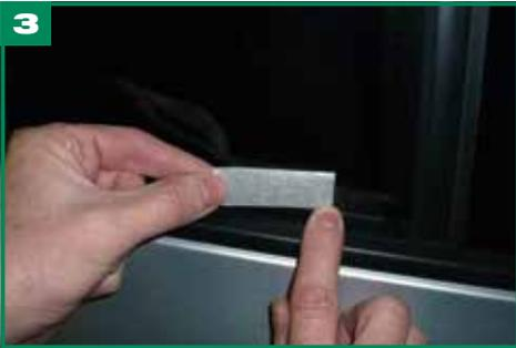
Apply stencil with printed VIN **shiny side** down to the glass. A wicking of the activator should occur and will vacuum down the stencil to glass. Adjust stencil placement if needed. Check the right position of the stencil! (whether VIN on the stencil is not upside down).
