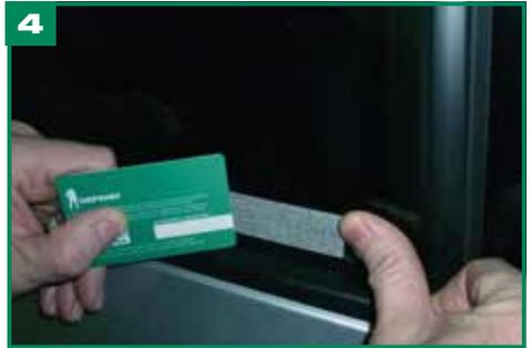
Force out remaining air and activator (e.g. by plastic card). **Now, let the remaining activator evaporate from glass and stencil.** This stencil mask is now secured to the glass. If light pressure forcibly moves the stencil, take off stencil and start over step 1.
