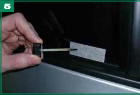
Brush 2 coats of etching gel DEFEND VIN.PRO.TEC (bottle marked as “step 3”) on top of the activated stencil so that all numbers and letters are covered.
