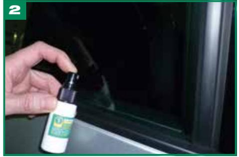
Spray glass with stencil activator 2 – 3 times (bottle marked as “step 1”). **Quickly move on to next step.** Do not let activator evaporate.
